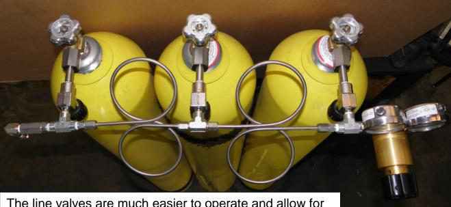
The line valves are much easier to operate and allow for easy servicing without depressurizing the tanks.
